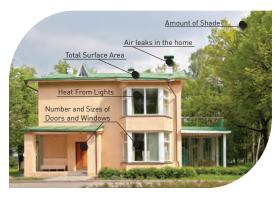
The proper selection of a Furnace, Air Conditioner or Heat Pump system is based on the heat gain, and/or losses from your home.
